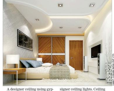
sum plasterboard takes anywhere from one to two weeks and can be completed in as much time or faster than a paint job. The major advantage of the plasterboards in designer ceilings over conventional ceilings (without false ceilings) is the smooth and undulation-free finish.
